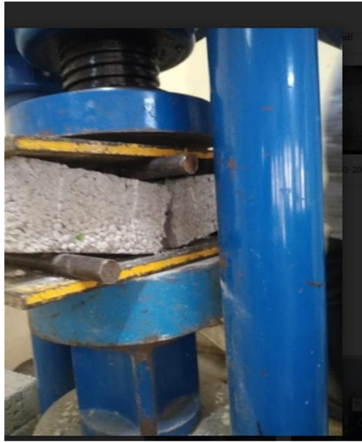
Fig 1: Flexural failure of concrete block
